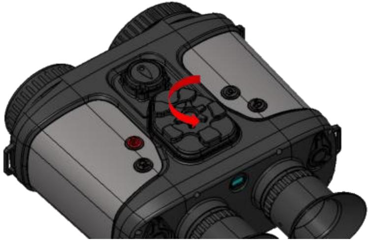
Step 2: Turn the battery cover knob counterclockwise, pull open the battery cover, insert the battery with the negative terminal facing upward.
