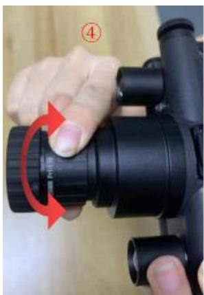
environment is visible, completing the objective lens adjustment. When observing targets at different distances, the objective lens must be readjusted according to the aforementioned method.
